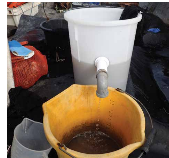
Figure 2.3: Equipment used to determine cultch availability via the water displacement method. (Photo: West Wales Shellfishermen's Association Ltd).
