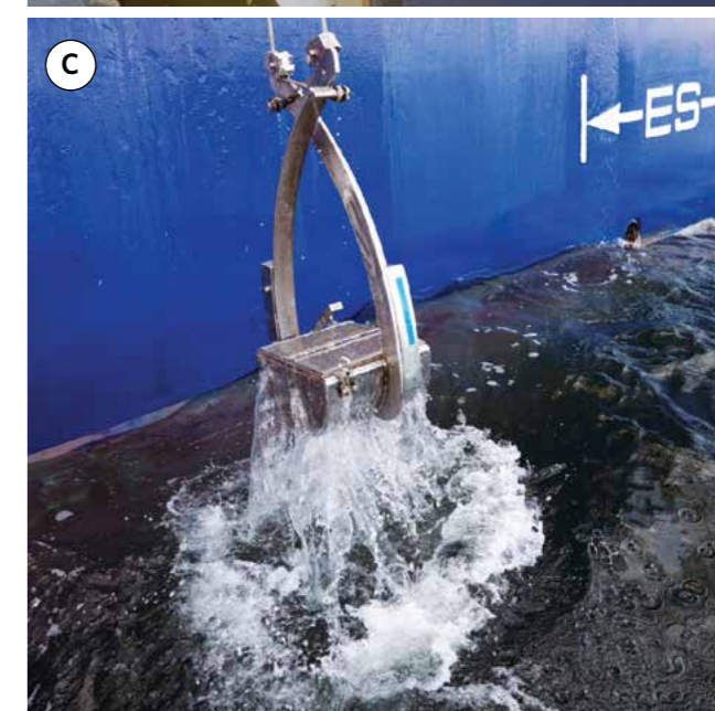
Figure 2.5: Grab sampler and box sieve. (Photos: Bernadette Pogoda).
